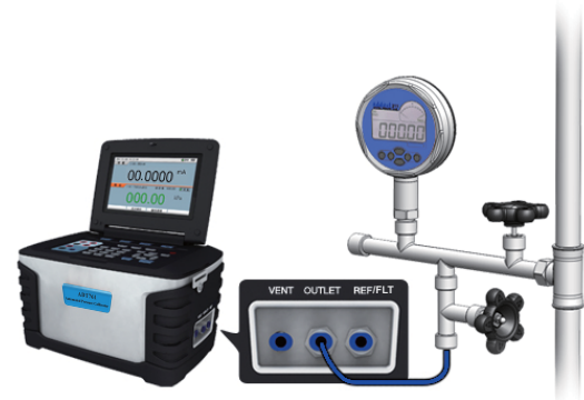
Figure 3-21 Calibrating a digital pressure gauge
