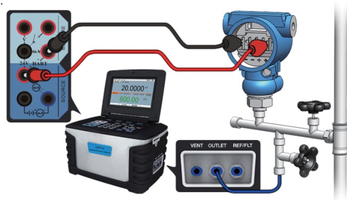
Figure 3-17 Calibrating a pressure transmitter
