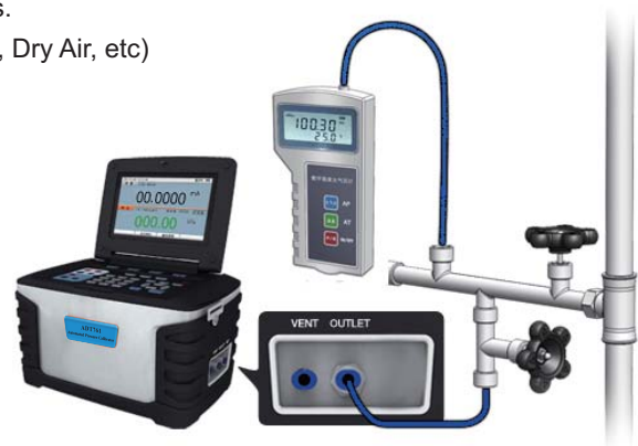
Figure 5-1 Calibrating a digital barometer
