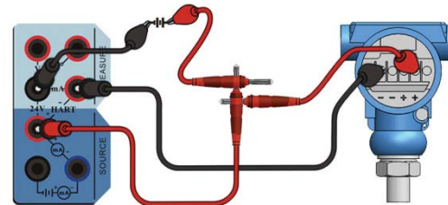
Figure 3-14 Internal series resistor and external loop power supply
