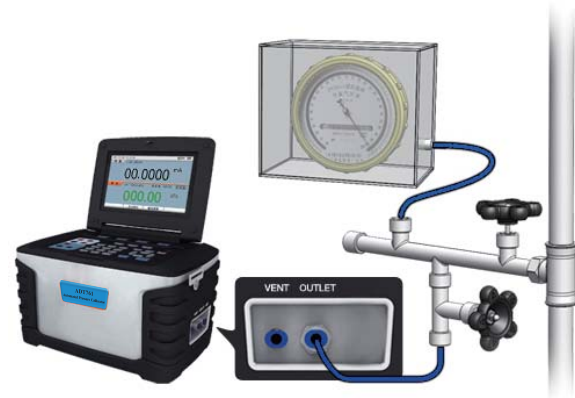
Figure 5-3 Calibrating an aneroid barometer
