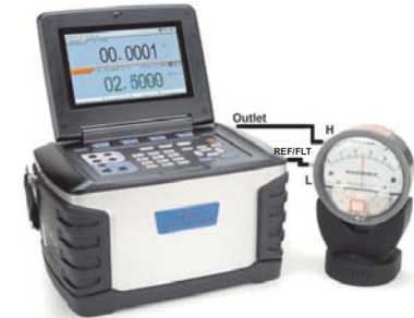
Figure 3-4 Differential pressure source
