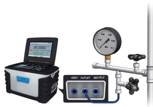
Figure 3-20 Calibrating a dial pressure gauge
