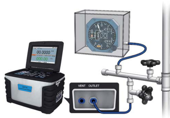
Figure 5-4 Calibrating a barometer altimeter
