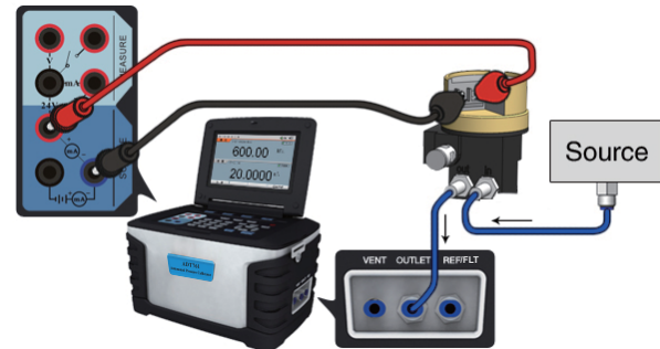
Figure 3-24 Calibrating an I/P converter
