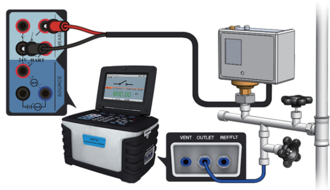
Figure 3-18 Calibrating a pressure switch
