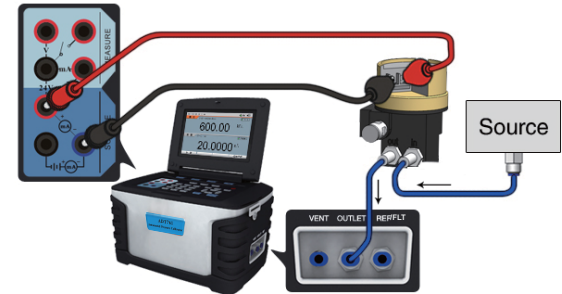
Figure 3-19 Calibrating a I/P converter
