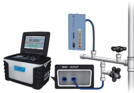
Figure 5-2 Calibrating a mercurial barometer
